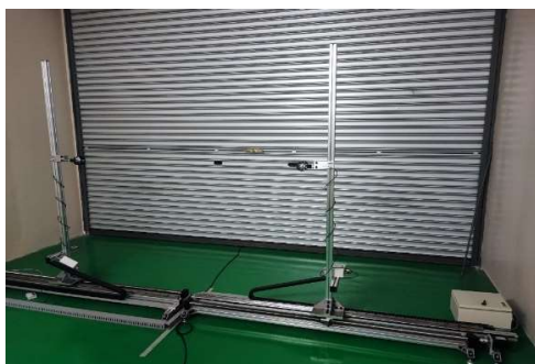
Air Delivery system for Table Fan with scada controller
