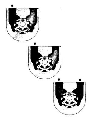
When the teeth mesh on the pressure side, the liquid is forced from the spaces and out through the discharge port.
