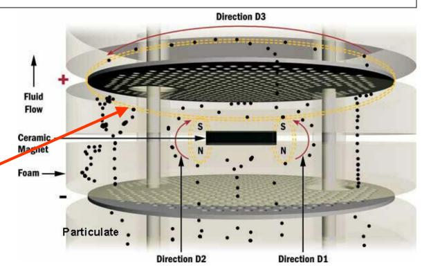
At the edges, other particulate forms a line, with half drawn upward, and half drawn downward
