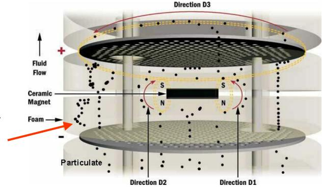
Some particulate "straws" itself into the foam, seeking an upward path
