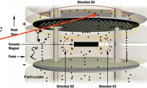
Repelled again by Coulombs force, particles move upward toward the next transition, or
