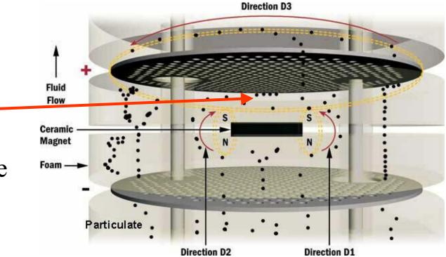
Some particles pass through the positive plate, reversing polarity
