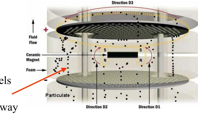
Coulombs force propels particulate upward, away from the plate
