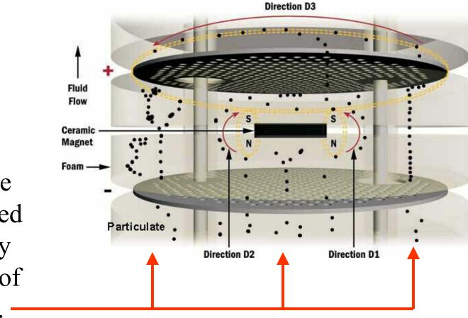
Particulate is propelled upward by the force of the pump. —
