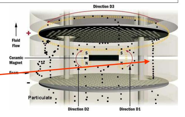
Other particles \_\_\_\_\_ stick to the positive plate and are held
