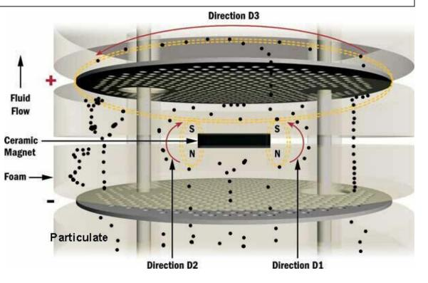
Uniquely, when the High Voltage is removed from the Cell, particulate falls toward the bottom, where it can be Backflushed out with shop air!
