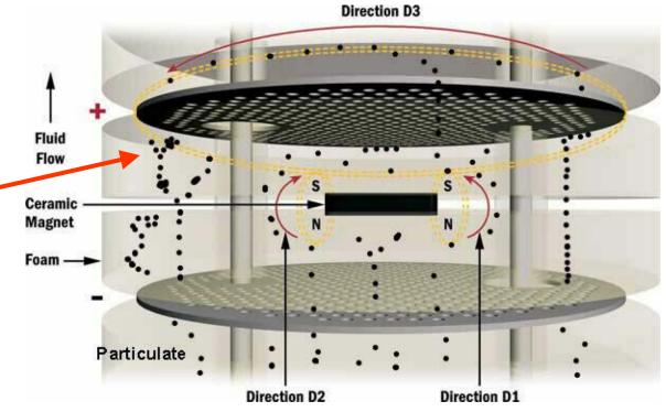
Particulate that is not trapped in the foam, or held in the force fields, continues upward, encountering three more like transitions
