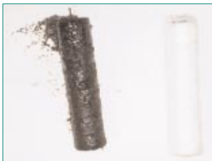
Photo 3. Shown are the fiberglass elements used in the HTF filters from Liquid Process Systems. On the right is a new unit and on the left is a used filter that has collected coke and other contaminants from a heat transfer system. The filter's housing consists of a filter with one of the fiberglass elements installed on a stand pipe designed to trap fine particles as small as 10 microns.
