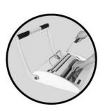
Loading comb ring, lifting the handle and opening the comb ring
