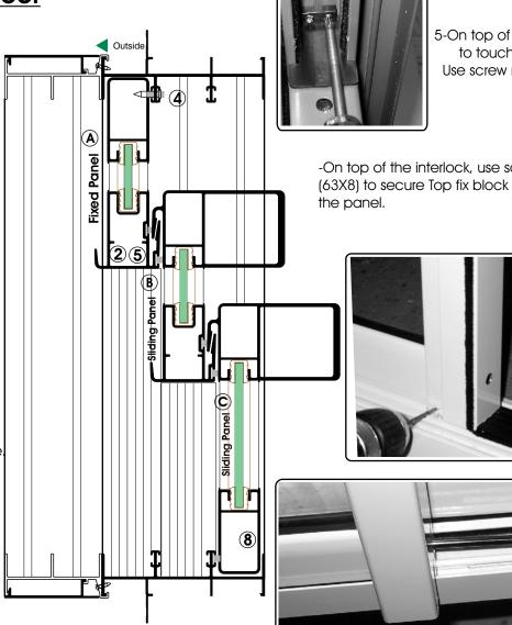
5-On top of the interlock, lift the Top fix block to touch the Head frame. Use screw (12X8) to secure it to frame.
