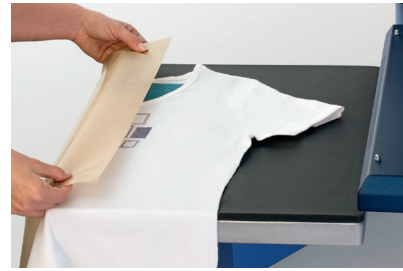
3 Make sure to apply the elements from the recommended side and use the correct pressurizing medium. To protect the heating surfaces from any glue residue, it is best to cover them with Teflon® film.
