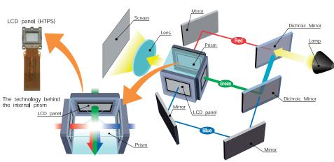
3LCD projector : RGB are projected at the same time, which makes the single composite image easy on the eyes
