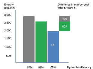
$Q_{\text{nom}} = 7 m^3 / \text{hour} \mid 8.760$  operating hours per year  $\mid 30$  mwc pressure  $\mid \in 0,15$  per kWh
