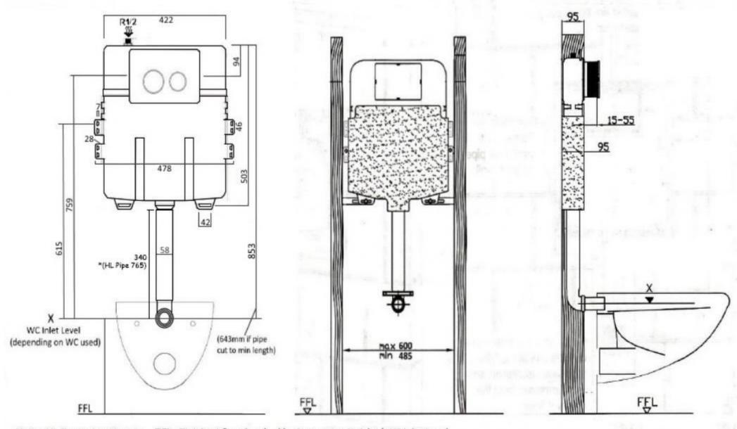
Note: All dimensions in mm; FFL=Finished floor level; X= Connection Height / WC Inlet Level.
