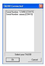
A list of all TAUSB / TA2USB connected to the PC will be shown. For each of them the Serial Number and the serial virtual channel assigned by Windows to the instrument will be indicated.
