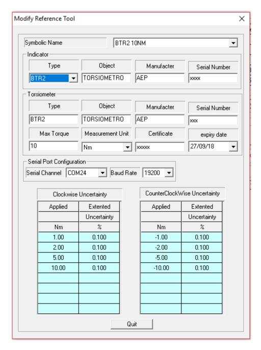
On this page are stored all data on the reference instruments that can be used during the calibration.
