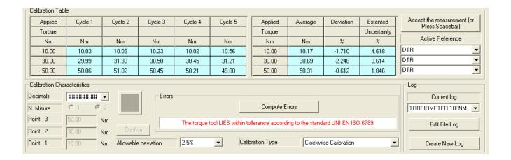
The number of measurement series of each torque value is 5
