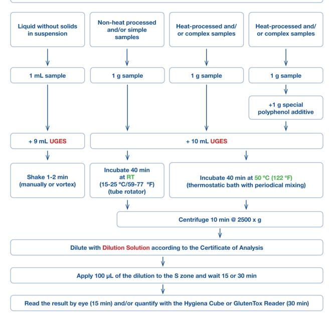
Figure 1. Scheme of use for GlutenTox Sticks Plus for Reader
