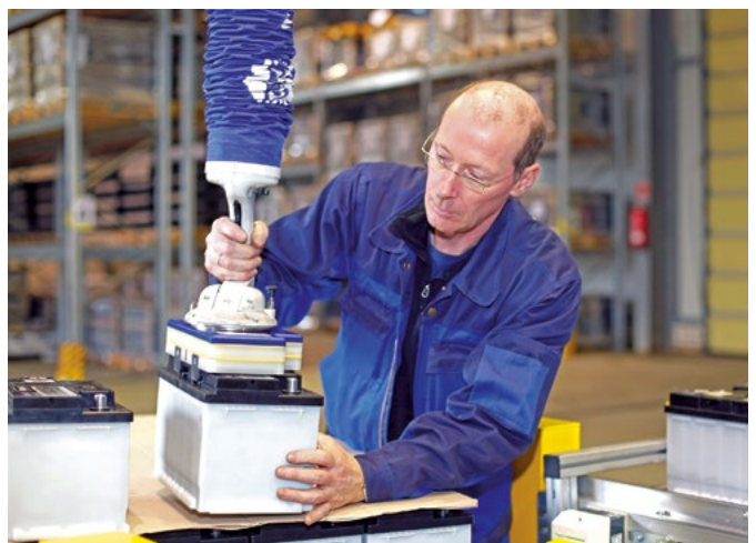
Vacuum tube lifter JumboFlex Battery for handling batteries
