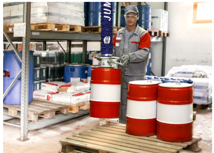
Vacuum tube lifter JumboSprint for handling barrels
