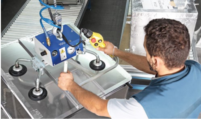
VacuMaster Light for handling metal housings
