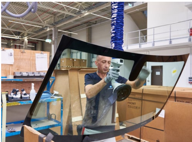
Vacuum tube lifter JumboFlex for handling windshields
