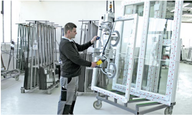
VacuMaster Window for rotating and palletizing windows
