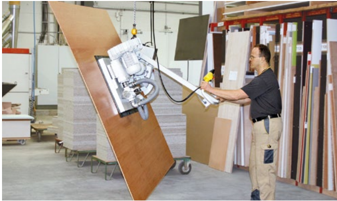
VacuMaster Multi for swiveling wooden boards by 90°
