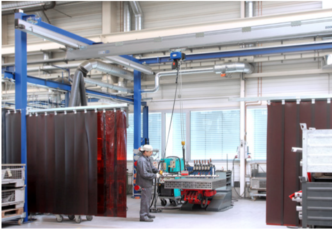
Aluminum single bridge crane system with reinforced section and a conductor line used with a chain hoist and a magnet
