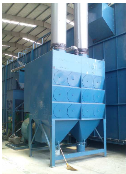
Typical Top Down Ducted Inlet to Collector Shown is Model 3DF24
