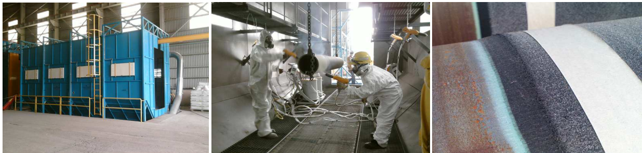
Spray Booth is immediately after the heating oven & the result is the 3 Layer Polyethylene/Polypropylene finish
