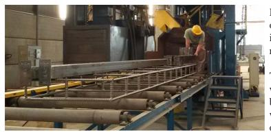
In case of handling work pieces that is of odd shape withour a flat bottom, that is preventing free movement along the roller conveyor, use a carrier.
