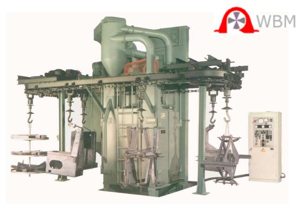
Many items can be blast cleaned most efficiently when hanging on a rotating hook. To achieve this Weblast has designed and engineered the finest monorail equipment. Rotoblast monorail designs use a series of work hooks suspended from an overhead trolley conveyor. The Conveyor can moves in either two speed pattern or moves in indexing manner.
