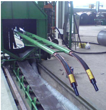
Long angle multiple nozzle blasting for pipe size between diameter from 12'' to 30''
