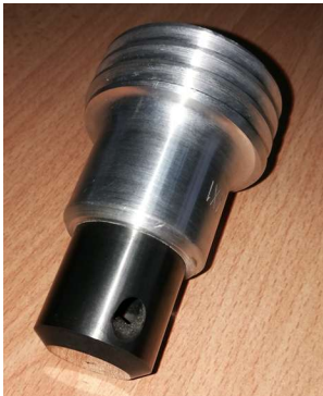
An angle nozzle for straight mounting in a rotated pipe blasting set up
