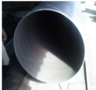
The pipe finishes appear clearly in spirally mark in rotated blasting
