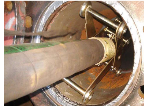
Circumferential cone shape blast stream for straight in & out blasting without having the pipe rotated, The centering guide is not needed in case of mounting with stiff blast lance.
