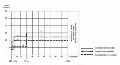
Figure 17: Limits for short-time vibration (Circulaire 23/07/86)
