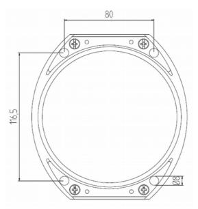
Figure 77: Dimensions of the mounting holes
