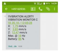
Figure 49: Example of received SMS message
