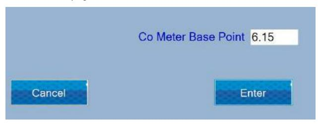
The operator enters the values of the buffer that will be used for calibration. Selection of buffer and principles of working with the system for measuring conductivity are described in the document WLS-TechManual. Pressing the Enter key passes to the actual calibration of the measurement system. Reports of this process is displayed in the System Status, in the upper right corner of the screen. By pressing the Cancel button procedure is terminated and transferred to the main screen.
