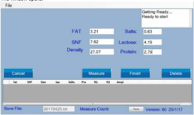
Input the parameter values for the high sample. By pressing the "Measure" button start a measurement
