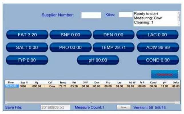
After the cleaning cycles are finished, the analyser returns "Lactoscan Cleaned" message and "Ready to start"
