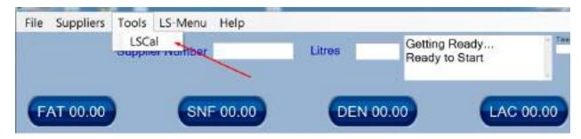
It opens the software tool for calibration. The operator chooses the Com Port, and presses the button Start. After that inputs the parameter values in the fields. With the button Measure starts a new measurement of the sample in calibration mode.
