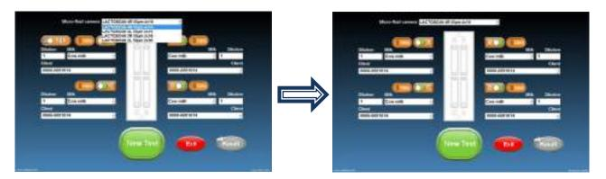
3. All the micro fluidic chambers of the LACTOCHIP are selected. If you want to use only 1 or 2, using button deselect the chambers which you will not be using in this test.
