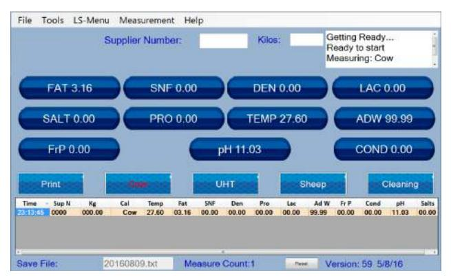
If there's serial printer connected (loaded with paper, with closed cover), the results are printed out. The analyser is ready for the next command (it is in Idle mode) i.e. ready for the next measurement. Button Print is active – by pressing it a copy of the results can be printed out (it is advisable one printout to remain in the milk collecting center, while the second one to be given to the deliverer).
