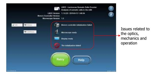
The issues may be caused by disconnection of cables, lack of power supply or software failure during the booting process. To eliminate them it is necessary to update the program by pressing the Retry button (try again).
