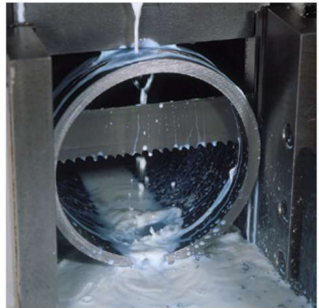
Start to cut material at reduced cutting rate.
