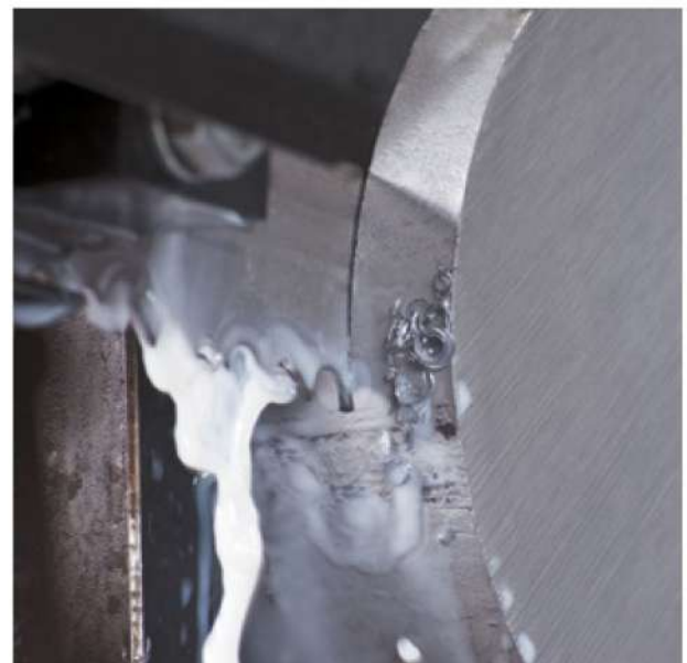
After break-in when the blade has fully entered the work-piece, increase the feed rate over series of cuts until the recommended cutting rate is achieved.
