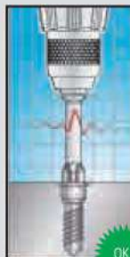
Common bit after impact test
