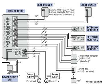
\*1 When you use an additional doorphone, the maximum number of the electric locks that can be connected to the doorphone depends on the type of doorphone. Consult your dealer for further information For VL-V554 users:
