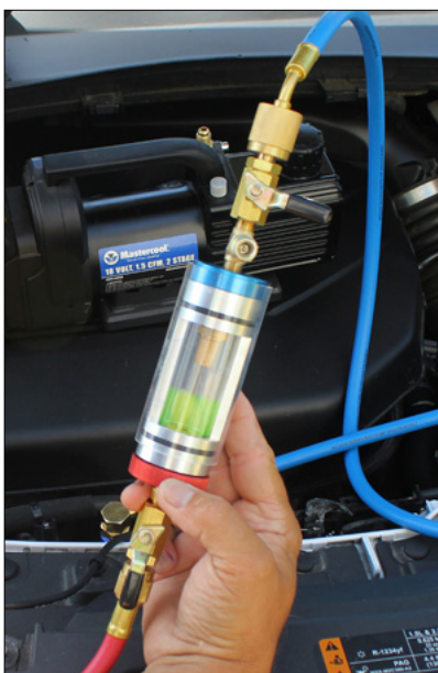
53377 R134a Visual Inspection Sight Glass with R134a Manual Couplers
