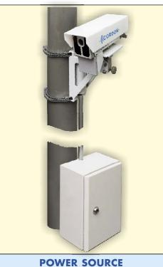
The system is installed on the roadside at height of 3-5 meters using the mounting bracket on any lighting pole or similar support. The mains power supply is not required, as the system is powered by replaceable battery in tamper-proof housing.
