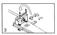
UNSCREW THE HOLDING SCREWS THEN REMOVE THE SCRAP COVERS AND HANDLE STOPPER.
