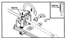
REPLACE THE SCRAP COVER MARKED AS 'L' ON SIDE MARKED AS 'L' ON BODY & SCRAP COVER MARKED AS 'R' ON SIDE MARKED AS 'R' ON BODY. ASSEMBLE THE PUNCHING MACHINE BACK TO THE ORIGINAL CONDITION PUSH THE COVER DOWN UNTIL IT GETS LOCKED WITH A CLICK.
