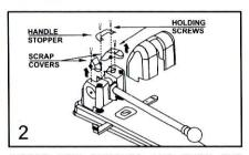
INSERT NEW PUNCHES AND TURN THE HANDLE TO FRONT SIDE WHILE KEEPING EQUAL HIGHT OF PUNCHES & PLACING TEETH TOWARDS BACKSIDE.
