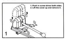
TURN THE HANDLE FULLY BACKWARD AND PULL THE WORN-OUT OR BROKEN PUNCHES OUT.
