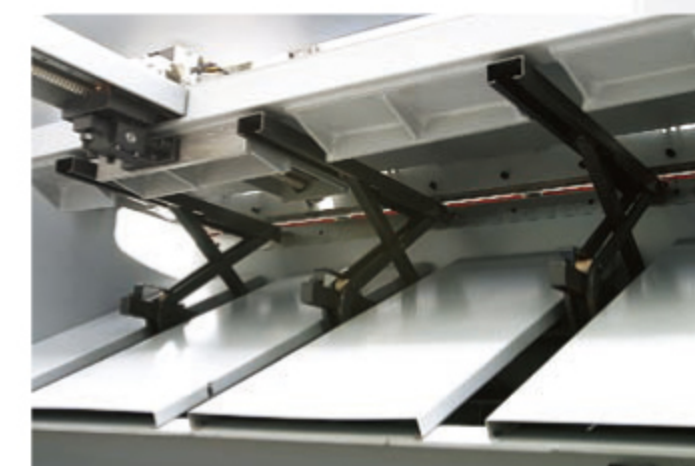
Squaring and/or support arms with extra long length (optional) Bras d'équerage et/ou de support extra longs (optionnel)
