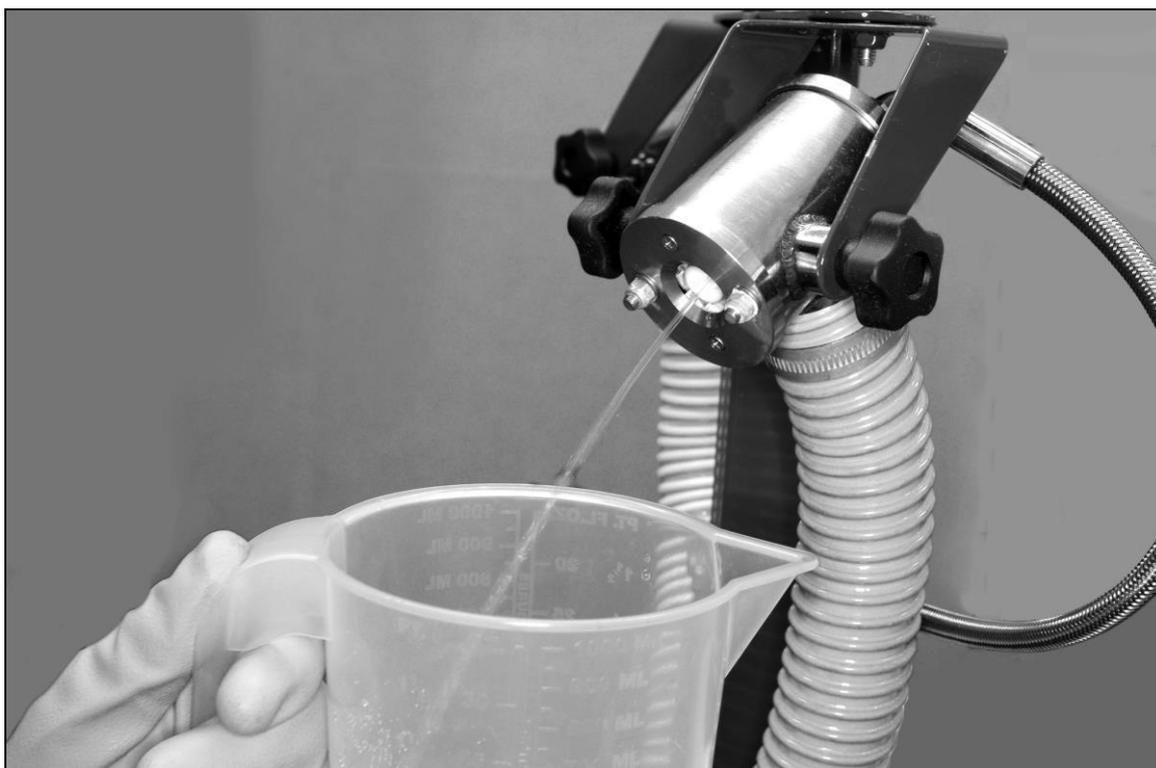
*Fig. 5 – Flow Calibration Check*
