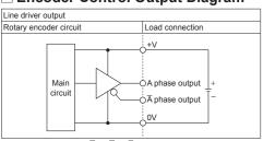
$\times$ All output circuits of A,  $\overline{A}$ , B,  $\overline{B}$ , Z,  $\overline{Z}$  phase are the same.  $\times$ The above specifi cations are subject to change and some models may be discon
