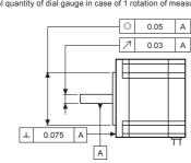
X3: Amount of radial shaft displacement when adding a radial load (25N) to the tip of the motor shaft.
