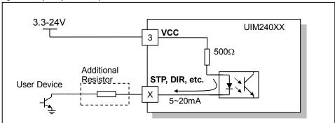
Note, in most situations, VCC can also be used as common cathode connection. This is because the opto-isolators used in UIM240 are bidirectional (AC&DC) type.
