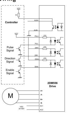
Remark:\* VCC is compatible with 5V or 24V; R1(3~5K) must be connected to control signal terminal.
