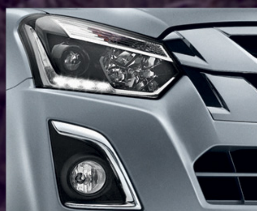
Projector Ellipsoid System Headlamps with integrated Daytime Running Lights
