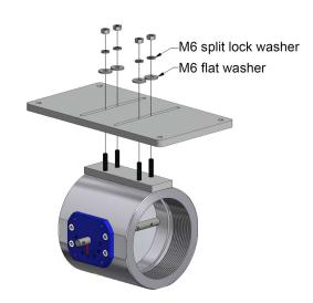
Figure 3: Actuator Mounting Bracket Installation
