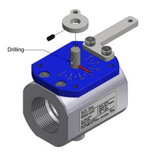
Figure 3: Crank Arm Installation
