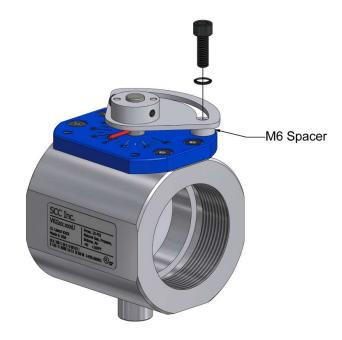
Figure 3: Completed Installation of AGA92.2 Manual Kit
