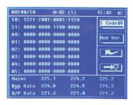
The status of all the key components inside the UPS can be monitored and displayed on the UPS panel, this function makes the maintenance of the system as simple as possible. Each bit on the figure represents the status of one component, it's easy for the maintenance people to identify the faulty component when there is a module or system fault.
