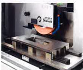
Special Jigs for warped work-pieces
