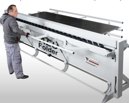
• The locking and folding feet are completely adjustable and are made of plastic that will not mark or scratch the surface of the composite panel during the bending process, even when folding of all four sides.
