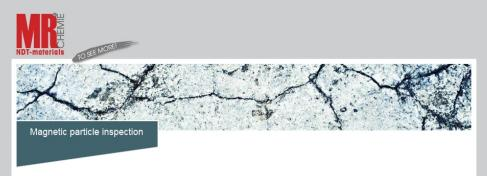
Magnetic particle inspection is suitable for detecting discontinuities (e.g. cracks) in or near the surface of ferromagnetic mate-rials.
