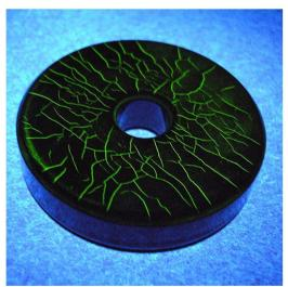
The magnetic powder is suspended in a carrier fluid. The particle size of the powder is smaller so that smaller discontinuities may be detected.
