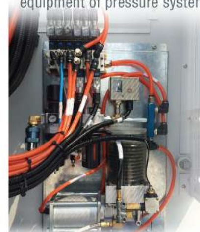
LUBRICATION AND PRESSURE SYSTEM
