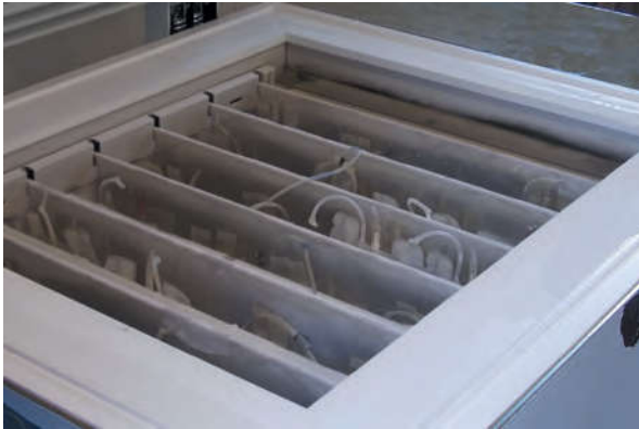
Internal case of the rapid freezer with standard 450 ml. bags in freezing
