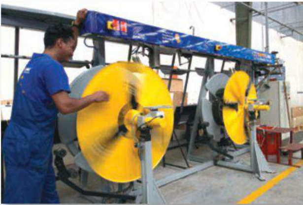
Manufacturing coils on the Buteline Pipewinder
