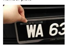
\*\* Please DO NOT place the sticker on metal surface or near any metallic object. Metal will severely inhibit reading range.
