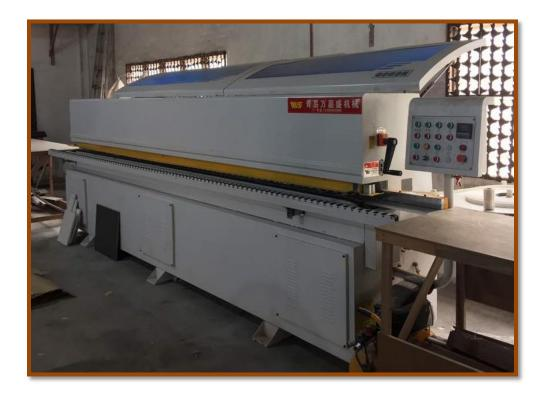
We use ABS Banding Machine's are to make a perfect finishing of PVC and ABS edges, after trimming unit working. When using the flat edge of the tools, the unit can also work as Glue –Scraper.
