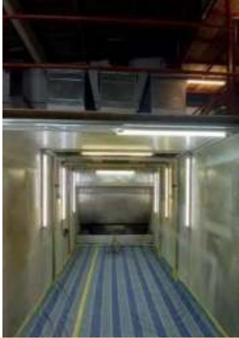
Dust Free Spray Booth- Water Curtain Filtering System
