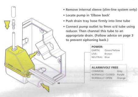
Wire the Mini Lime Pump to the permanent Live, Neutral and Earth terminals of the Evaporator. Install a 1.0 amp in-line fuse between the Mini Lime Pump and the Evaporator.
