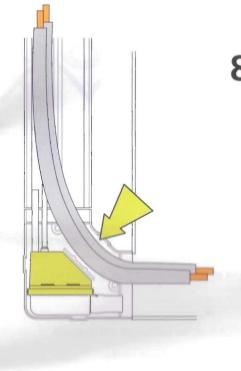
Slide 'Internal sleeve' (slim-line system only) into place and clip 'Elbow front' and 'Conduit front' into position.
