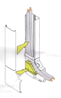
**9** Remove backing and push 'Ceiling plate' into position.
