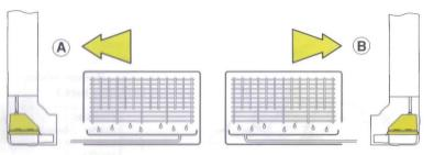
Disassemble system. Hold 'Elbow back', 'Internal conduit sleeve' (slim-line system only) and 'Conduit back' against the wall, squaring up to the ceiling and the evaporator unit. Drill fixing holes in wall and secure using rawl plugs and screws supplied.
