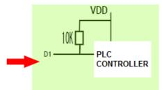
Recommendation: Please connector a 10k resistor to every channel output as above diagram to provide stable output to the controller.
