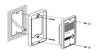
After attaching the body supporter with 2screws, put the indoorstation into the grooves of body supporter, and then fix it with screws.
